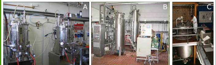
Bioreactors for production of bacterial-feeding nematodes in liquid media: A - lab scale (12 liter), B - pilot scale (500 liter), C - production plant (3,000 liter). All facilities at e~nema GmbH (Schwentinental near Kiel, Germany)
